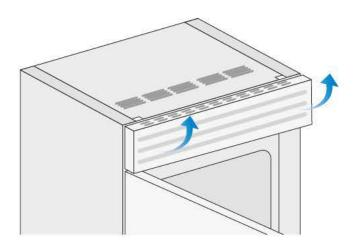
> Clean the condenser thoroughly from all dust deposits as shown in the figure, taking care not to damage it.
