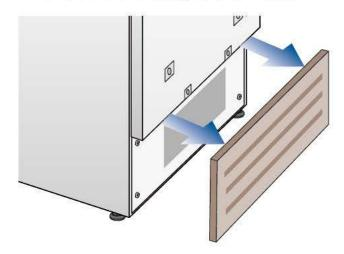
> Clean the condenser thoroughly from all dust deposits as shown in the figure, taking care not to damage it.
