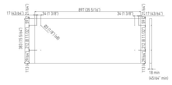
**Integrated Panel Recommendations** Panels with thickness ranging between 18 mm and mm. Panels with weight max of 12 kg. Provide installation of decorative panels during installation of the unit.
